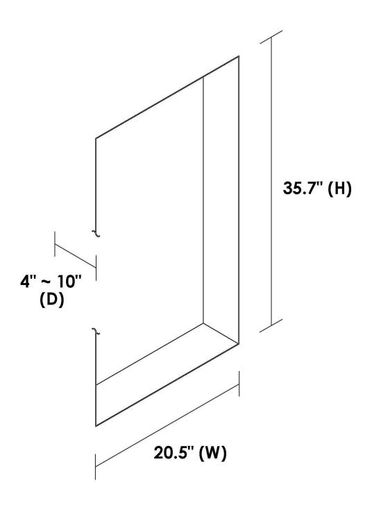
The maximum wall thickness for installation is 10". If a wall thickness of less than 4" will be used, then you will need to fabricate a spacer to fill the distance between the back of the wall and the side brackets.
