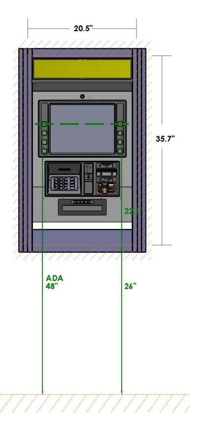
The outside dimensions of the GT5000 are shown below, the 24" X 38.5" dimension represents the machine with the front bezel installed.
