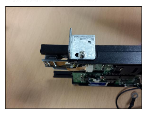
With both brackets installed as shown, you're ready to install the assembly to the back of the bezel.
