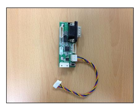
Connect the reset board to the 9-pin serial port on the side of the ATM motherboard. Use the two machine screws included with the kit.
