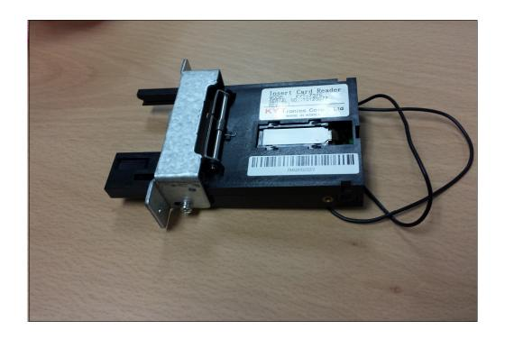
Using the 2 course-thread screws included with the kit, install the new reader assembly into the back of the card reader bezel.
