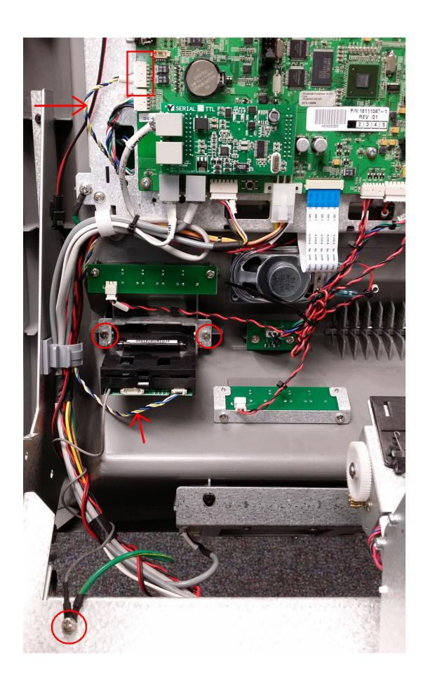
Once the cable is freed up, remove it from the ATM completely along with the card reader. You will not reuse either of these.
