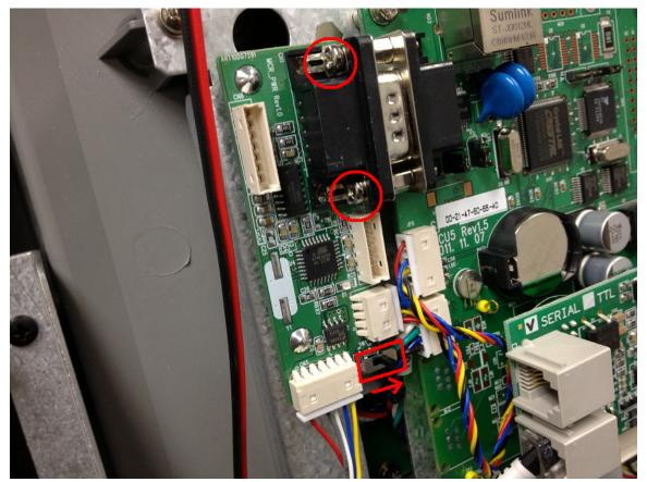
Plug the jumper wire (red, blue, yellow, black) in as shown above, the wires will be tight, so route them down under the modem so they do not get pinched. Attach the card reader wire to the bottom.
