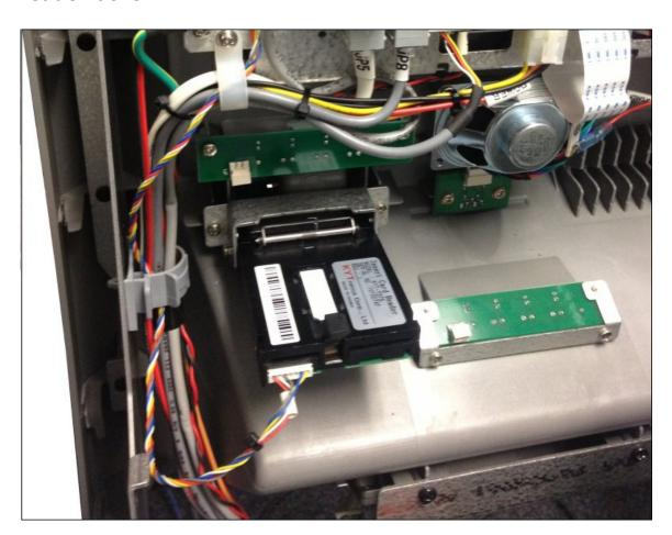
When you install the new card reader, we recommend leaving the screws a little loose, and then try inserting a card in from the front. The card should slide in and out easily without hanging up on the bezel.
