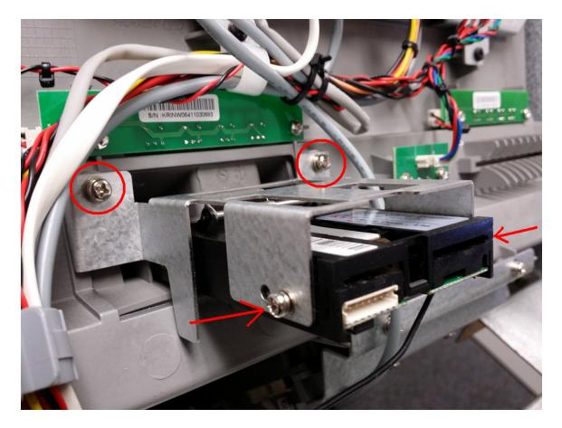
Next you need to prepare the reset board. Plug the jumper wire included in the kit into the reset board as shown below.
