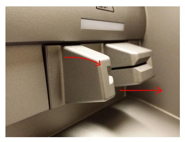
Prepare the new EMV reader. Attach the new card reader brackets using the old card reader to bracket screws or the ones in the kit if you lost the originals. Refer to image below.
