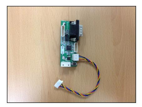
Connect the reset board to the 9-pin serial port on the side of the ATM motherboard. Use the two machine screws included with the kit.
