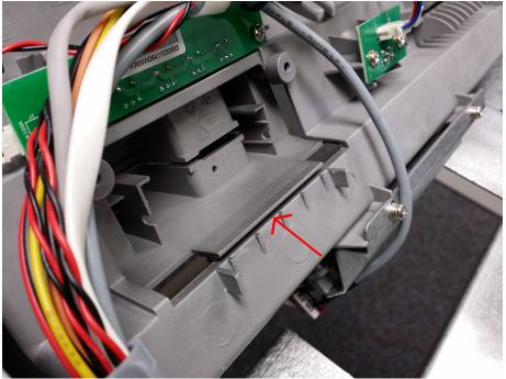
Once you have the bottom tab lined up, push the card reader bezel forward and it should lock into place. If it's not going in properly, refer to the image below on how the front should line up.
