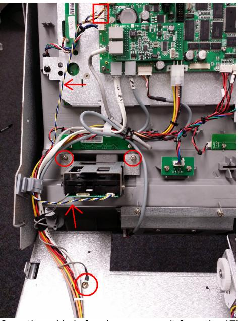
Once the cable is freed up, remove it from the ATM completely along with the card reader. You will not reuse either of these.
