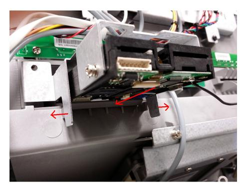
Once you have it sitting in there properly, use the bracket to bezel screws included with the kit to secure the bracket to the card reader bezel (red circles). See below image. Do not tighten them yet.
