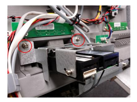
Now wrap the ground cable to the wiring harness and reattach the ground cable to the sliding tray as shown below.
