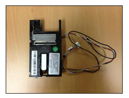
Card reader bracket (1) with card reader mounting screws (2) And card reader bracket to bezel screws (2)
