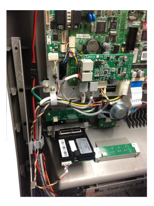
There is a small jumper included with the kit. To install, you must first identify which type of motherboard you ATM is using. ACU-3 or ACU-5
