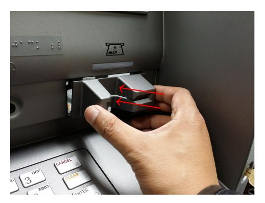
Pay attention to the tab on the bottom rear of the card reader bezel. It should sit inside the main bezel as shown below.
