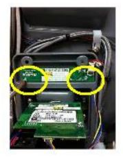
3. Remove the 4 screws that hold the card reader bezel and remove the card reader with bezel.
