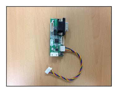
Reference image below. Connect the reset board to the 9pin serial port on the side of the ATM motherboard. Use the two machine screws included with the kit. Refer to red circle for screw points. Note the small switch (red rectangle) on the reset board, it goes to the right.
