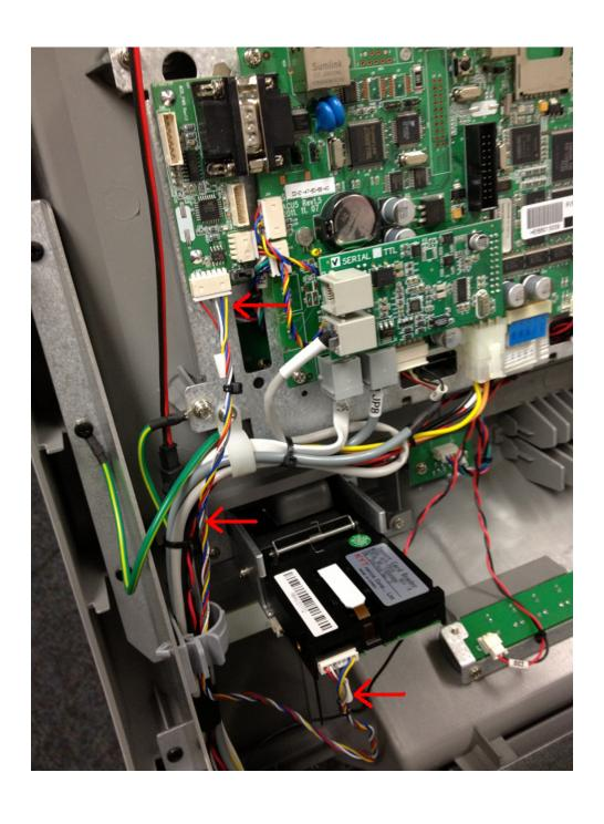
There is a small yellow jumper included with the kit. To install, you must first identify which type of motherboard you ATM is using. ACU-3 or ACU-5
