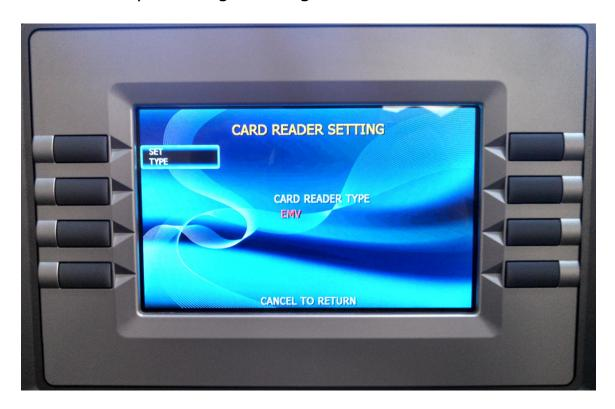
Once this has been set, return the ATM to normal operation and dip your card and remove to test and verify that it's operating normally.
