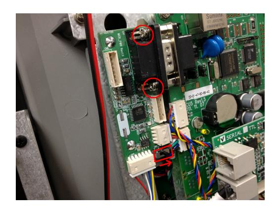
Plug the jumper wire (red, blue, yellow, black) in as shown above, the wires will be tight, so route them down under the modem so they do not get pinched. Attach the card reader wire to the bottom.
