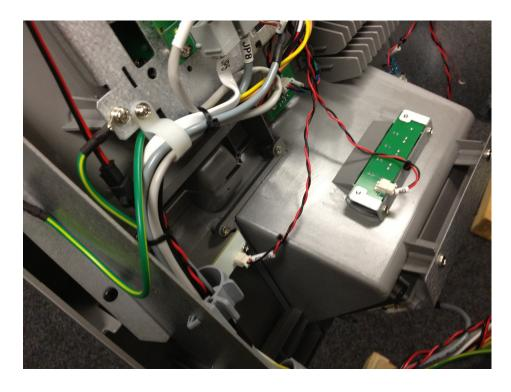
Attach using the old screws and connect the red/black wire to the back of the 'flicker' or LED light panel.
