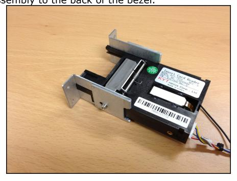
Using the 4 course-thread screws included with the kit, install the new reader assembly into the back of the card reader bezel.
